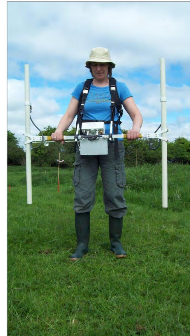
Geophysics in action. The above picture shows a fluxgate magnetometer being used. This piece of equipment measures the magnetic field of archaeological features, such as anything that has been burnt or baked, like a fireplace (hearth).
