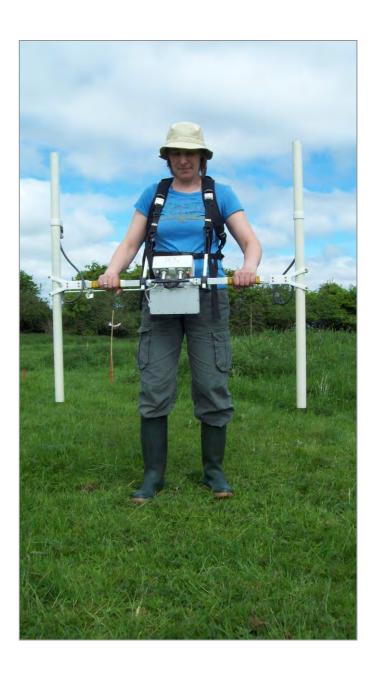
Geophysics in action. The above picture shows a fluxgate magnetometer being used. This piece of equipment measures the magnetic field of archaeological features, such as anything that has been burnt or baked, like a fireplace (hearth).
